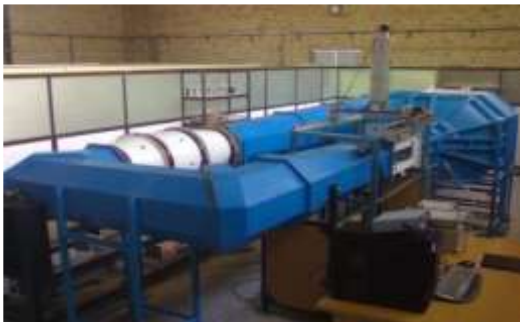
Fig. 4- Closed-circuit wind tunnel used in the research.
